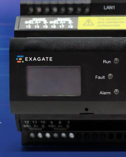
Battery Monitoring Systems (BMS) are essential for maintaining the optimal performance and lifespan of batteries used in diverse applications, including UPS systems, data centers, telecommunication base stations, and solar energy storage units. These systems feature intelligent monitoring capabilities designed to track the health, status, and performance metrics of individual batteries and battery groups.
